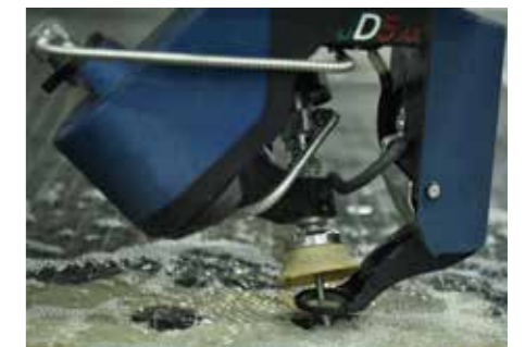
New Z axis strokes up to 350 mm 3-axis and up to 200 mm 5-axis and tube cutting up to ø 500 mm (std)
