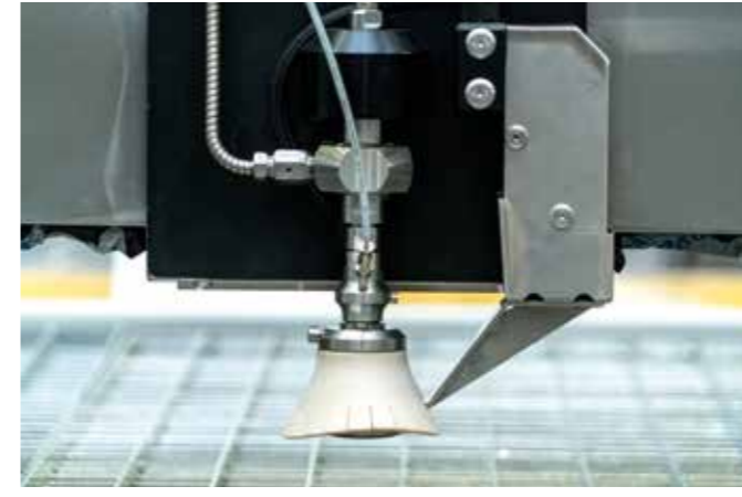
PROBE Probe system, continuous or periodic, available also with large ring for foam or glass cutting. It enables to maintain the same distance from the material being cut at all times even if the material is not perfectly flat.
