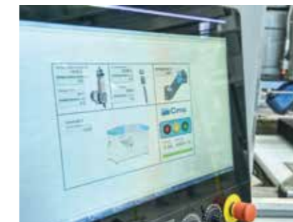
Hardware and software for the waterjet cutting system designed to offer simple and userfriendly management of all system functions, including conicity control (JDC) for 5-axis machining centres
