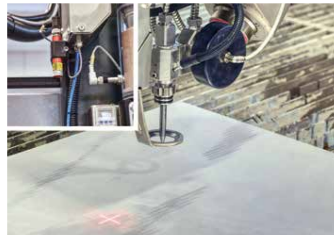
Cross Laser device for setting one or multiple starting point on the sheet positioned on the cutting table (opt).
