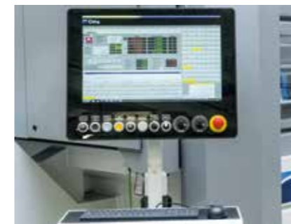
Hardware and software for the waterjet cutting system designed to offer simple and userfriendly management of all system functions, including conicity control (JDC) for 5-axis machining centres
