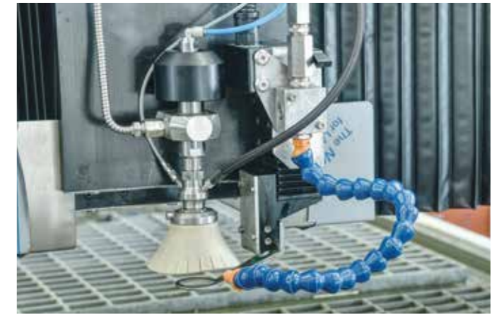
Cleaning system for the work area which reduces the chances of scratches on the cut piece. It also enables the feeler to detect correctly the thickness of the material (opt).
