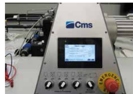
Software-based electronic control of cutting pressure
